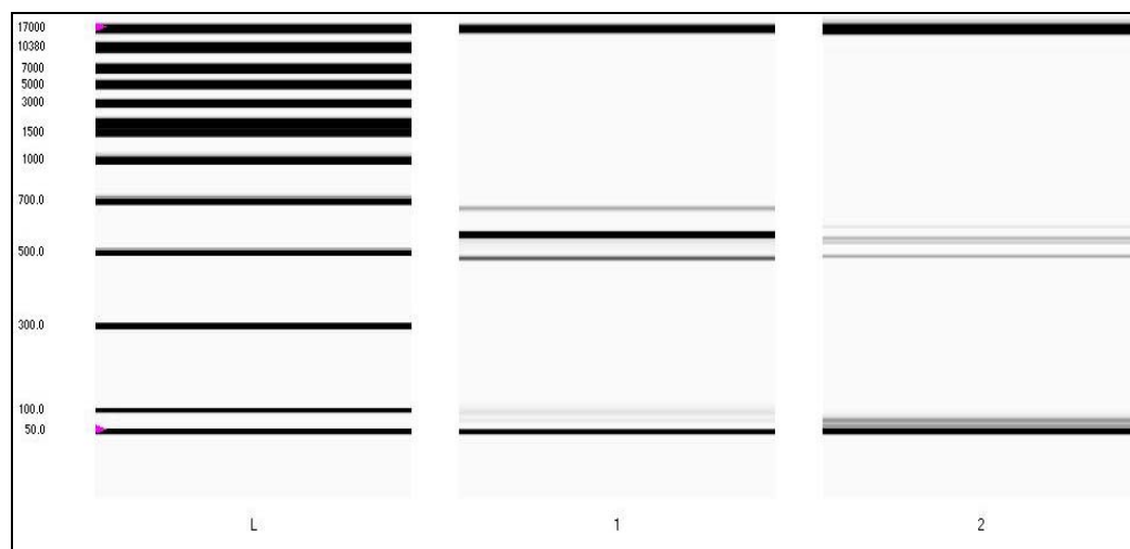
Figure 3.24 Capillary electrophoresis gel. Comparison between PCR products, produced with Plant-A1/A2 primers: 1) soya leaves and 2) soya oil.
