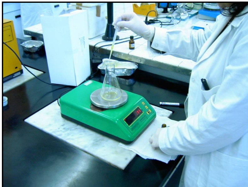
Figure 20: Weighting of 2g of oil in 250 ml conical flask by the mean of an analytical balance.
