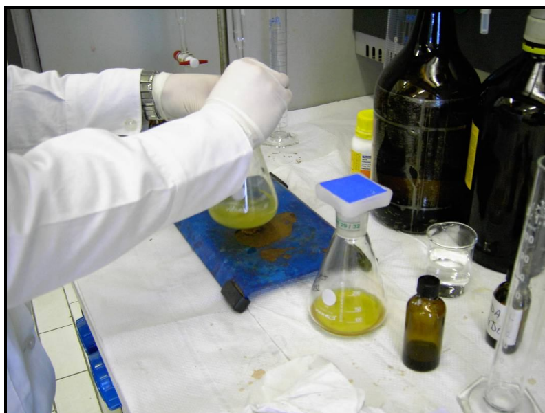
Figure 21: Titration step for the determination of peroxide value.
