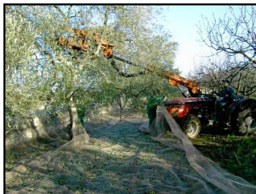
Figure 13: Trunk vibrator provoke olives fall on the net covering ground.
